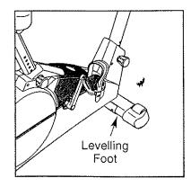
both of the levelling feet under the front stabiliser until the rocking motion is eliminated.
