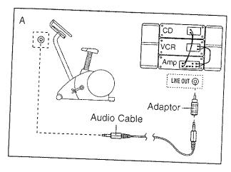
B. Plug one end of the audio cable into the jack beneath the console. Plug the other end of the audio cable into the adaptor. Plug the adaptor into an RCA Y-adaptor (available at electronics stores). Next, remove the wire that is currently plugged into the LINE OUT jack on your stereo and plug the wire into the unused side of the Y-adaptor. Plug the Y-adaptor into the LINE OUT jack on your stereo.
