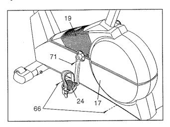
Using an adjustable wrench, turn the Left Pedal (24) clockwise and remove it. Next, remove the two Screws (66) from the Left Side Shield (17). Remove the Screw (71) from the left side of the Side Shield Cover (19) and lift it off. Gently remove the Left Side Shield.
