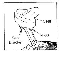
turn the indicated knob counterclockwise two or three turns to loosen it (if the knob is not loosened enough, it may scratch the seat bracket). Next, pull the knob, slide the seat to the desired position, and then release the knob. Move the seat bracket forward and backward slightly until the pin on the knob snaps into one of the holes in the seat bracket. Then, turn the knob clockwise until it is tight.
