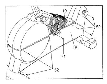
Remove the seven Screws (52) from the Right Side Shield (18). Next, remove the Screw (71) from the right side of the Side Shield Cover (19).
