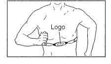
sensor unit as described above. Adjust the length of the chest strap, if necessary. The chest pulse sensor should be under your clothes, against your skin, and as high under the pectoral muscles or breasts as is comfortable. Make sure that the logo is right-side-up and facing forward.
